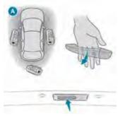
With the electronic key in recognition zone A, pass your hand behind the door handle of one of the four doors or press the tailgate opening control.
